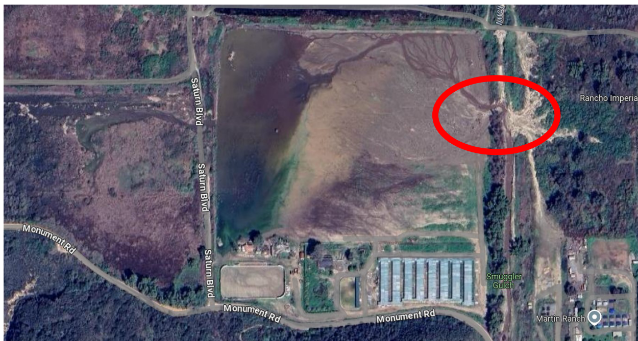
Image 8 – Smuggler's Gulch Pilot Channel breach and flooding of adjacent property
